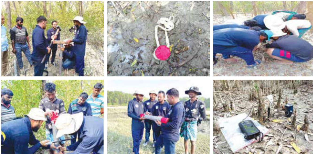
Figure 02: Soil core sampling process of blue carbon ecosystem in the deltaic coast of Bangladesh (Hatiya, Noakhali)
