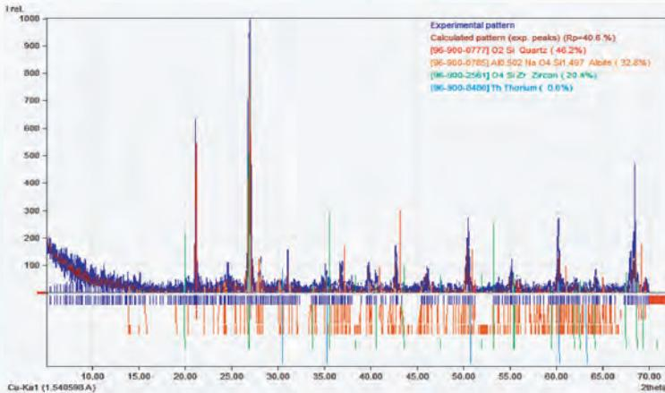
Figure-3: XRD peak of a sample showing the presence of Zircon & Thorium.
