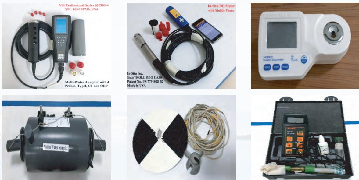
**Figure 2:** (a) Multi-water analyzer (YSI Professional Series-626909-4, Made in USA); (b) In-Situ DO meter (SmarTROLL RDO CA30, Made in USA); (c) Seawater Refractometer (HANNA: HI 96822); (d) Niskin Water Sampler (Hydrobius, Made in Germany); (e) pH Meter (HANNA: HI 8424) and (f) Secchi Disc
